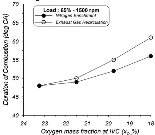
**FIGURE 9A.** Duration of Combustion as a function of oxygen mass fraction of the inducted mixture, at 1500 rpm and 65% load, for (i) NEIM and (ii) EGR operating modes.
