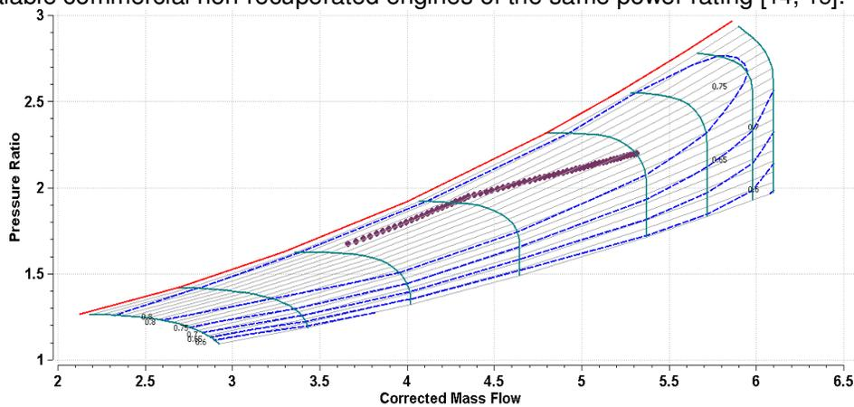
FIGURE 4: LP Compressor Map and Operating line
