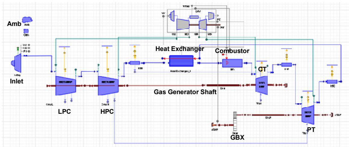
**FIGURE 9:** Recuperated Turboshaft engine PROOSIS schematic diagram
