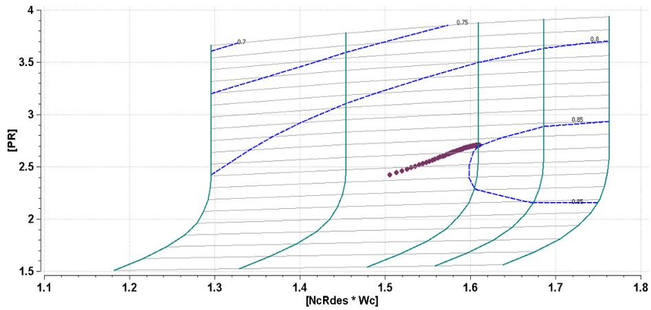
FIGURE 6: Core Turbine Map and Operating line
