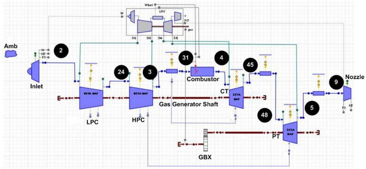
**FIGURE 3:** Turboshaft engine PROOSIS schematic diagram & station numbering
