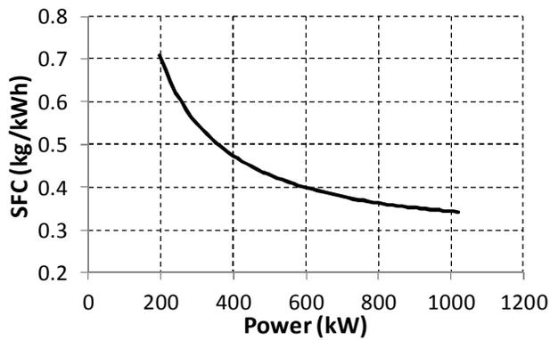
FIGURE 8: Engine sfc-power performance curve
