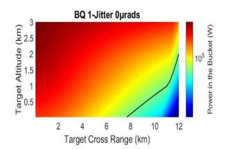
**Figure 13.** Contour Plot for Altitude versus Range. This plot refers to the ideal situation where beam quality is perfect and we have zero platform jitter. The effective range of the HEL is indicated by the contour line, which indicates the PIB threshold estimated earlier.
