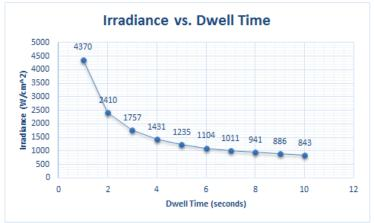
FIGURE 2. Estimated peak irradiance for a 3-mm thick aluminum sheet for various dwell times. Based upon the maximum laser dwell time, we can estimate the minimum value of peak irradiance required to melt the target.
