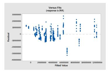
**FIGURE 6.** Versus fits plot for irradiance. The variance of the residuals is non-constant over the range of the fitted values and violates the second DOE assumption.
