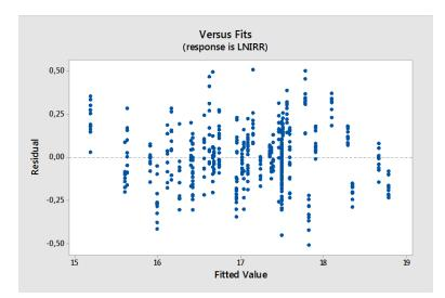
**FIGURE 8.** Versus fits plot for the transformed response. A natural logarithm transformation on irradiance appears to remove the issue of the non-constant variance of residuals.
