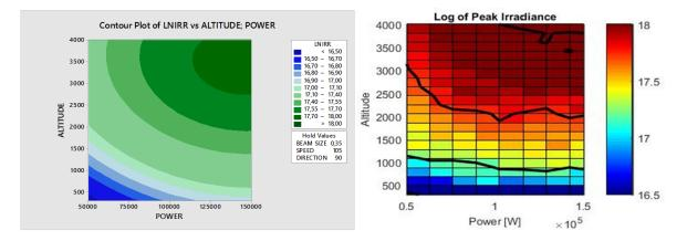
**FIGURE 10.** Model Comparison between Minitab and WaveTrain for the natural log of the peak irradiance on target. The main pattern of the contour lines, which is of most interest for this study, seem to follow the same trends as the ones from Minitab. Starting from a 50 kW power, it has a negative slope that, by the level of around 150 kW, has stabilized. Both plots also exhibit predict a similar spread in peak irradiances.
