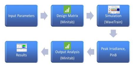
**FIGURE 4**. DOE Workflow. The statistical package Minitab was used for the experimental simulation design generation and the output analysis, whereas the full diffraction code, WaveTrain, was used for the laser beam propagation simulation. All WaveTrain simulations were executed by Dr. Pogue.
