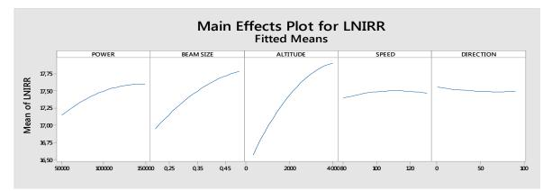
**FIGURE 9.** Main Effects plot for LN Irradiance for laser output power (in watts), beam director diameter (in meters), platform altitude (in meters), platform speed (in m/s), and platform direction (in degrees azimuth). Altitude has the most significant effect to the peak irradiance, followed by beam director size and power. Speed and direction seem to have only minor effects on the response.
