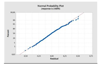
**FIGURE 7.** Normal Probability plot for the transformed response. A natural logarithm transformation on irradiance appears to alienate the issue of the non-normal distributed residuals.
