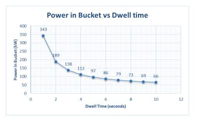
**FIGURE 3.** Power-in-the-bucket for a 3-mm thick aluminum sheet for various dwell times. Based upon the maximum laser dwell time, we can estimate the minimum value of PIB required to melt the target.
