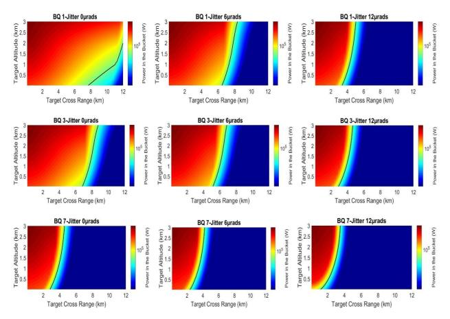
**Figure 14.** Platform Jitter and Beam Quality Effects. Starting from the upper left plot, which shows the ideal situation ( $M^2$ =1 and jitter=0), we see that the HEL's effective range is almost 8km. The lower right plot ( $M^2$ =7 and jitter=12µrad) shows the significant decrease of the effective range down to almost 1km.
