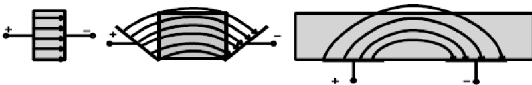
FIGURE 1. From the parallel to the coplanar capacitor configuration: the interdigital sensor and the resulting electric field.
