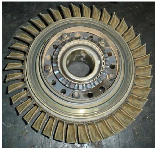
**FIGURE 3.** The gas generator turbine rotor with the blades positioned around the rotor disk. The cooling plates are fixed with five bolts on the rotor disk. Notice the sand-color of the blades.
