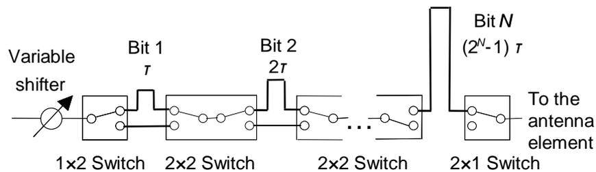
**FIGURE 3:** A typical  $N$ -bit switched time delay line network that requires  $N-1$   $2 \times 2$  switches to implement the  $2^N$  different time delay settings. Signal in each bit can follow either the delay or non-delay path; a microwave phase shifter provides the fine modulo- $2\pi$  phase control.
