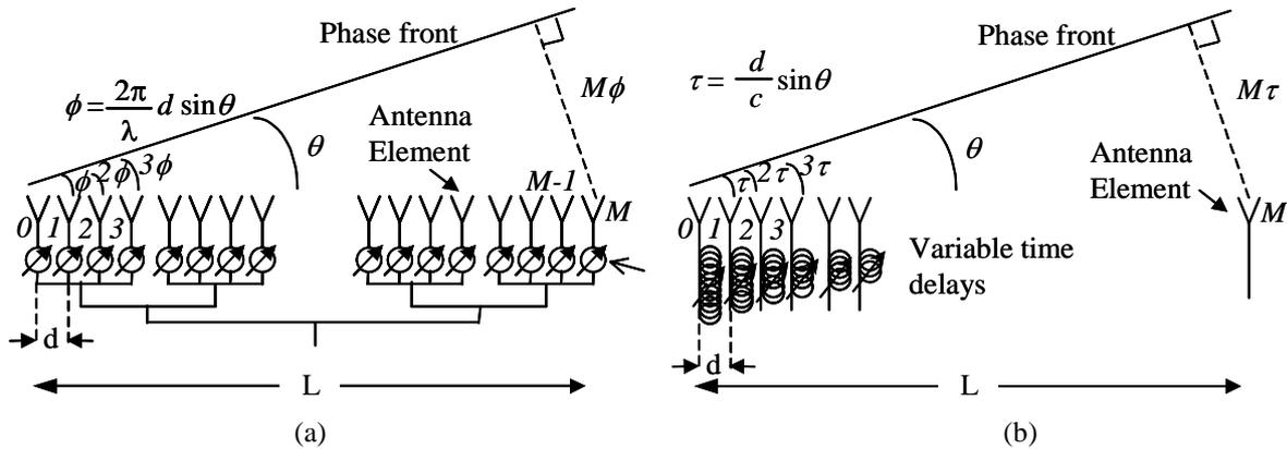
**FIGURE 2.** (a) Schematic representation of a phased antenna array with phase based control; (b) PAA with time delay based control. One dimension is shown for simplicity.
