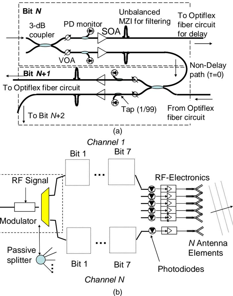
**FIGURE 6.** (a) Physical design of the elemental PDL, (b) The PDL system consisting of  $N$  7-bit Delays addressing  $N$  antenna elements.
