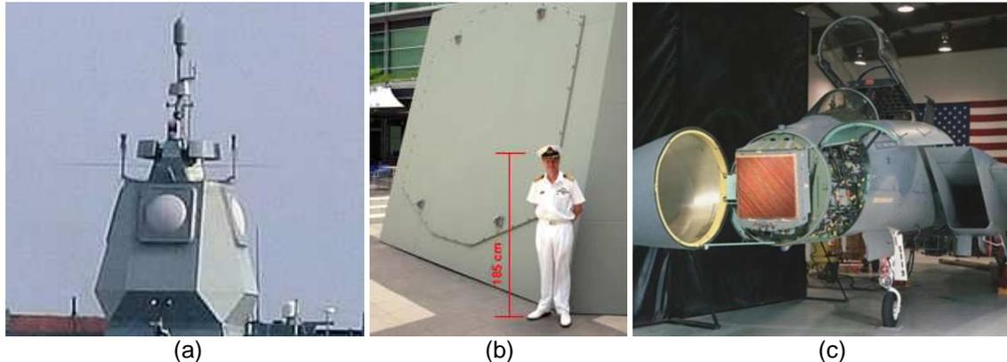
**FIGURE 1:** (a) Active Phased Array Radar mounted on top of Sachsen class frigate F220 Hamburg's superstructure manufactured by Thales Nederland [1]. (b) Aegis combat system in the USS Pinckney (DDG 91) [2].
